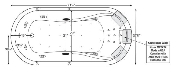
Numbered areas on tub deck represent possible locations to install cleaning systems, faucets and other fixtures.
